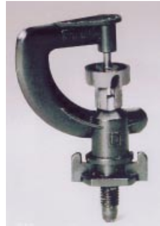
Figure 8. The spray system in this garden sprinkler was molded of Delrin® acetal resin for superior wear, UV stability, and the best properties for snap-fitting the sprinkler head. Courtesy of PLASTECH.
