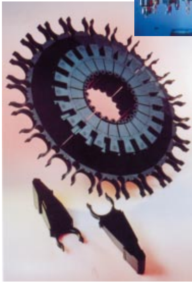
Figure 9. This tool changer carousel is comprised of 22 identical components made from Delrin® 100 acetal resin for the best balance of stiffness and strength coupled with flex fatigue resistance needed for the spring fingers of the tool gripper. Courtesy of Bridgeport Machines Ltd.
