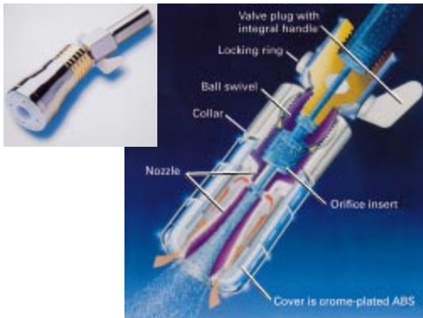
Figure 10. Six parts injection molded from Delrin® play key roles in water-saving spa™ 2001 Shower heads with adjustable spray and massaging action. Courtesy of Energy Technology Laboratories.
