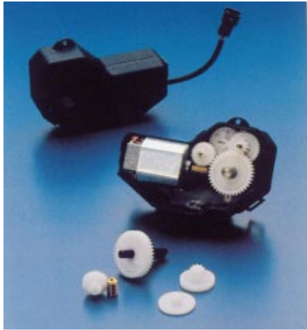
Figure 15. Delrin®100 gives a superior combination of stiffness and toughness as well as excellent dimensional stability in this motor and gearbox for automotive air conditioning control. Courtesy of Mikron A.G.
